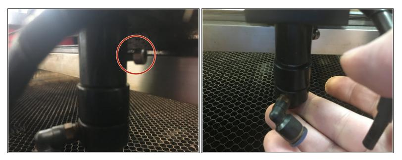
Locate the socket-head cap screw holding the lens tube into the mirror assembly.
