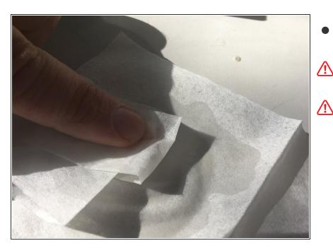
Use an alcohol moistened Kimwipe to clean both side of the lens.
