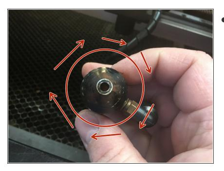
Screw the air assist nozzle back onto the lens tube.
