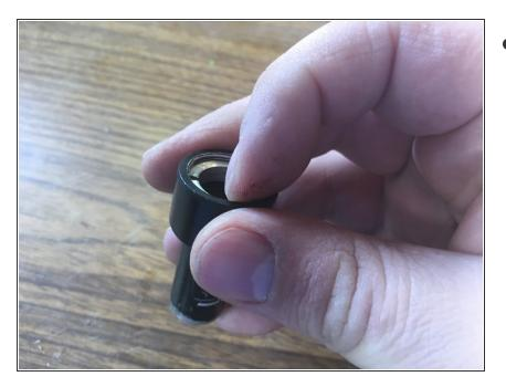
Use your finger to loosen and remove the lens retaining ring the rest of the way.
