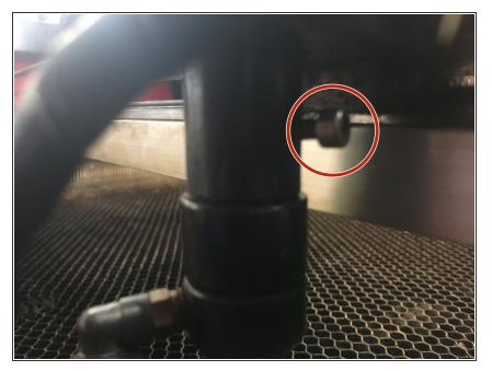
• Reinstall the lens tube and tighten the sockethead cap screw to hold it in place.
