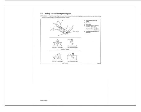
Welding wire is energized when gun trigger is pressed. Before lowering helmet and pressing trigger, be sure wire is no more than 1/2 in. (13 mm) past end of nozzle, and tip of wire is positioned correctly on seam.
