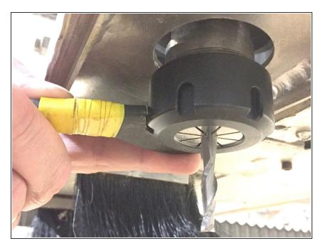
If performing a tool change, remove the existing bit, collet and collet nut from the spindle.
