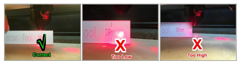
• Use the raise and lower buttons to move bed until focus tool just fits between the laser head and your material.
