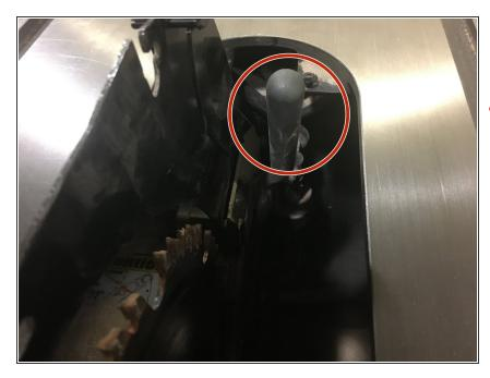
Rotate the locking lever down and toward the back of the machine.
