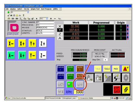
On the "Axes+Spindle Screen," click the "spindle stop" button.
