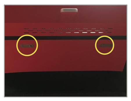
Open the door on the front of the machine by pressing the two latches.
