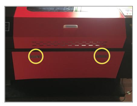
Close the chip door and secure the latches.
