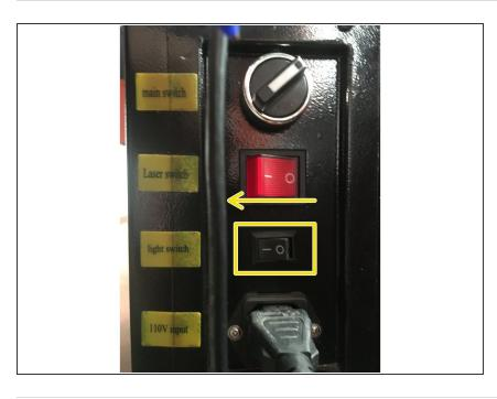
Turn the fluorescent work light ON by flipping the switch on the side of the machine toward the "I".
